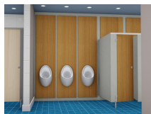
Urinals on service duct panels
