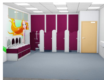
4 bay cubicles including one as ambulant compliant
