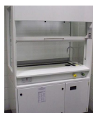
Re-circulation fume cupboard
